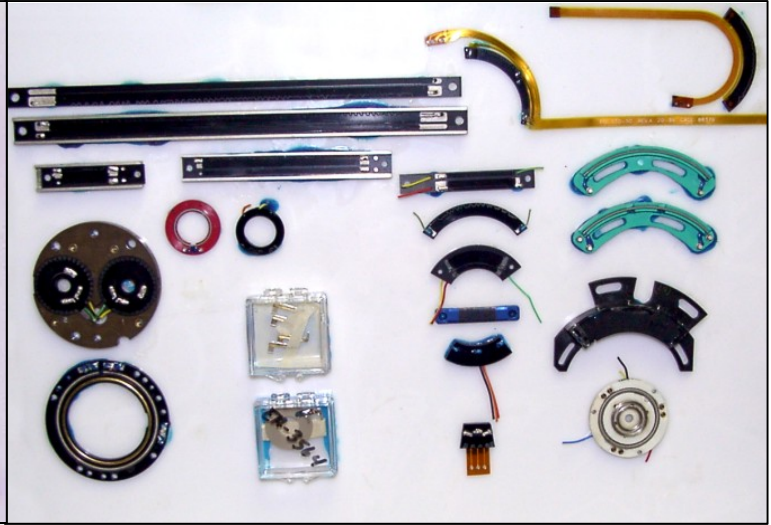
Conductive-Plastic and Wire-Wound elements
