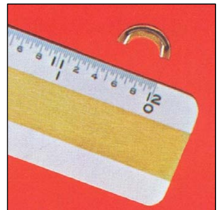
Miniature gyro pick-off element with scale to show actual size
